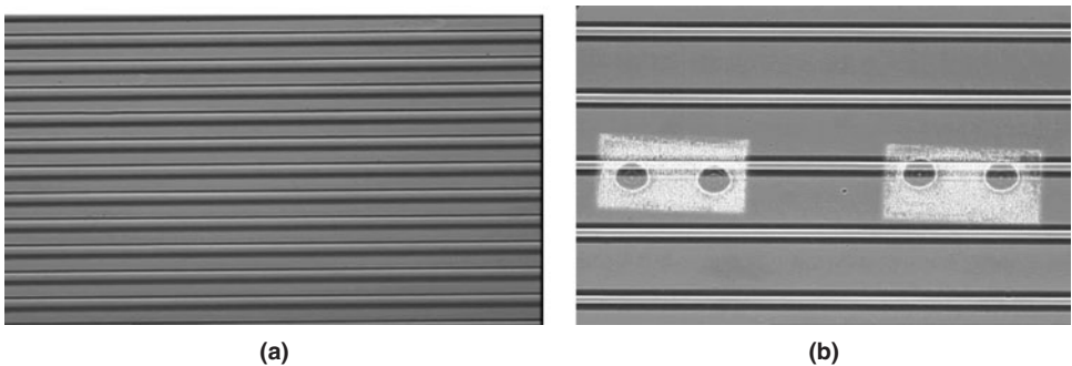
FIGURE 6.13 (a) Waveguide array with 10\text{ }\mu\text{m} wide \times 5\text{ }\mu\text{m} thick cores on a 20\text{-}\mu\text{m} pitch formed on a PCB. (b) Waveguide array ( 50\text{ }\mu\text{m} wide \times 25\text{ }\mu\text{m} tall cores on a 250\text{-}\mu\text{m} pitch) formed on a buffer layer over copper pads and microvias on a PCB.
