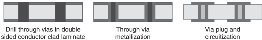
FIGURE 7.9 Process flow for an insulating core.
