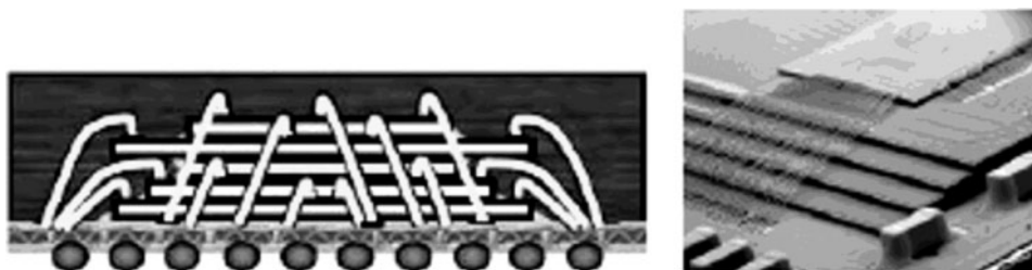
FIGURE 1.12 Three-dimensional integration using wire bonding.
